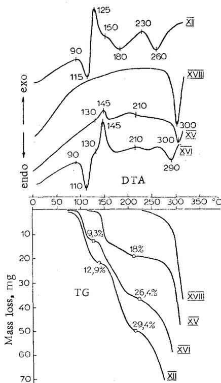
Fig. 1. Thermoanalytical curves (DTA and TG) of XII (sample weight 170 mg), XV (sample weight 100 mg), XVI (sample weight 140 mg), and XVIII (sample weight 90 mg).
